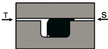
Elastomer damaged due to extrusion.
