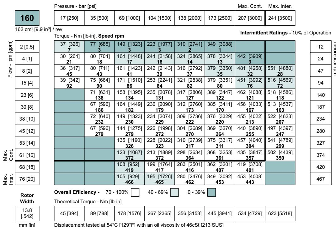
► Performance data is typical. Performance of production units varies slightly from one motor to another. Operating at maximum continuous pressure and maximum continuous flow simultaneously is not recommended. For additional information on product testing please refer to page 6.
