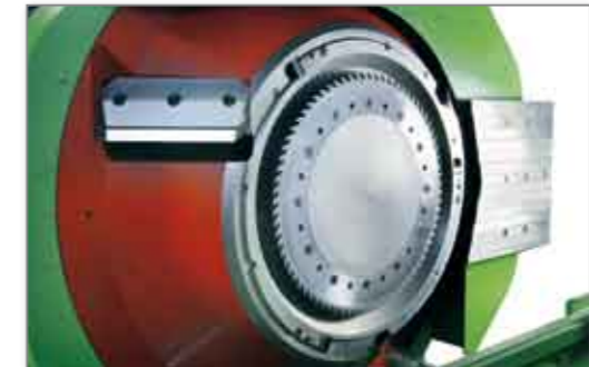
Straight knives chipper head with post-sawing circular saw ring for opening of the heads in the cut
