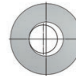
An eccentric shaft results in leakages at high speeds.
